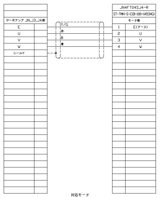
J4用: HG-KR053(B), HG-KR13(B), HG-KR23(B), HG-KR43(B), HG-KR73(B) HG-MR053(B), HG-MR13(B), HG-MR23(B), HG-MR43(B), HG-MR73(B) J3用: HF-KP053(B), HF-KP13(B), HF-KP23(B), HF-KP43(B), HF-KP73(B) HF-MP053(B), HF-MP13(B), HF-MP23(B), HF-MP43(B), HF-MP73(B) JN用: HF-KN053(B), HF-KN13(B), HF-KN23(B), HF-KN43(B)
