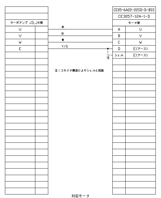
J4用: HG-SR121(B),HG-SR201(B),HG-SR202(B) HG-SR2024(B),HG-SR3524(B) J3用: HF-SP121(B),HF-SP201(B),HF-SP202(B) HF-SP2024(B),HF-SP3524(B)
