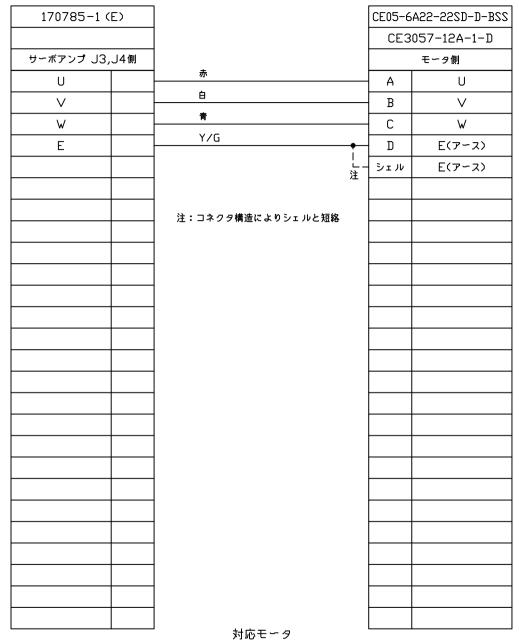
J4用: HG-SR301(B), HG-SR352(B), HG-JR353(B) J3用: HF-SP301(B), HF-SP352(B), HF-JP353(B)
